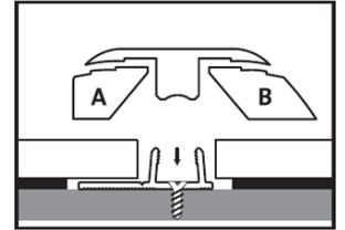
Saw the profile to the right length. Cut away section A and section B with the knife to make the expansion profile.
